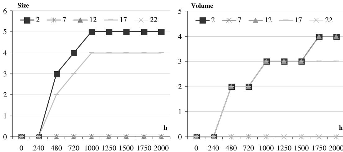
Fig. 4. MAG welding panels characteristics from degree of blistering according EN ISO 4627-2
