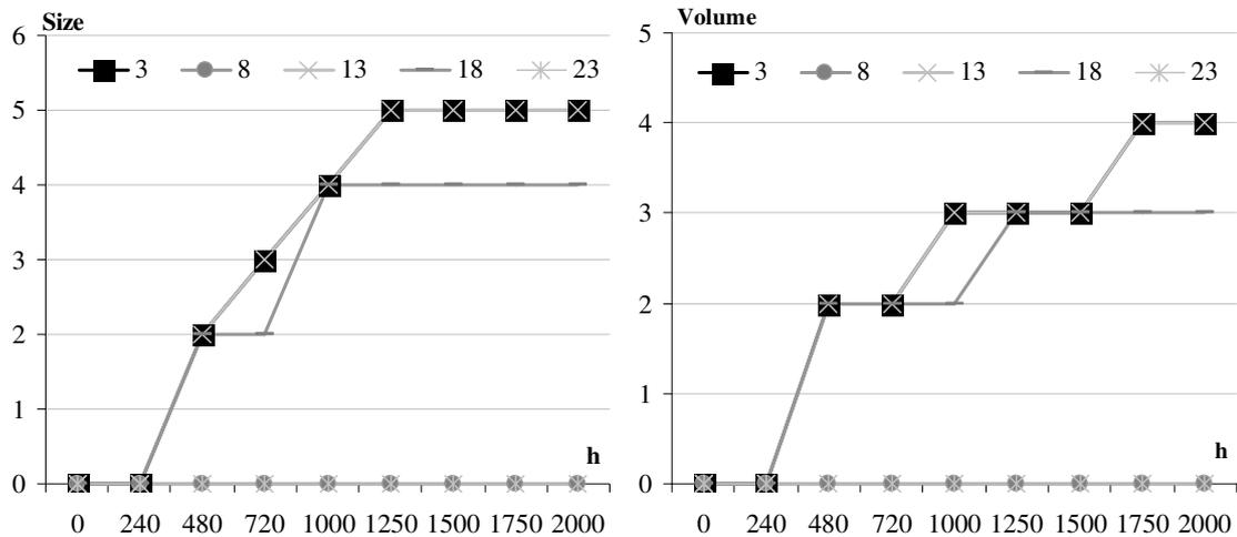
Fig. 1. Spot welding panels characteristics from degree of blistering according EN ISO 4627-2
