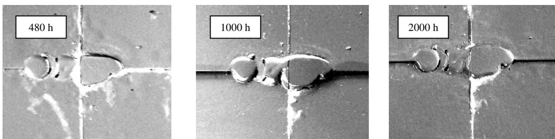
Fig. 6. Spot welding panels of Sample 2 – observation by 480h, 1000h, 2000h
