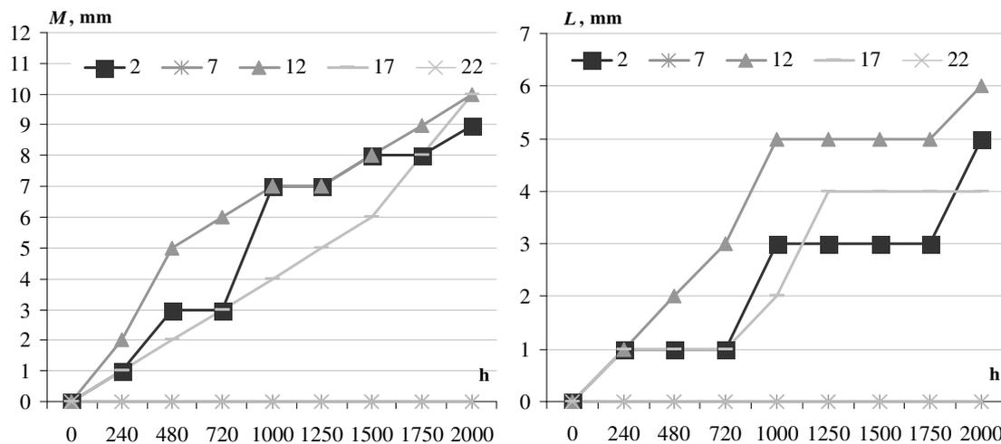
Fig. 5. MAG welding panels characteristics from degree of filiform corrosion - EN ISO 4627-10
