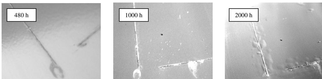
**Fig. 9. Spot welding panels of Sample 16 – observation by 480h, 1000h, 2000h**
