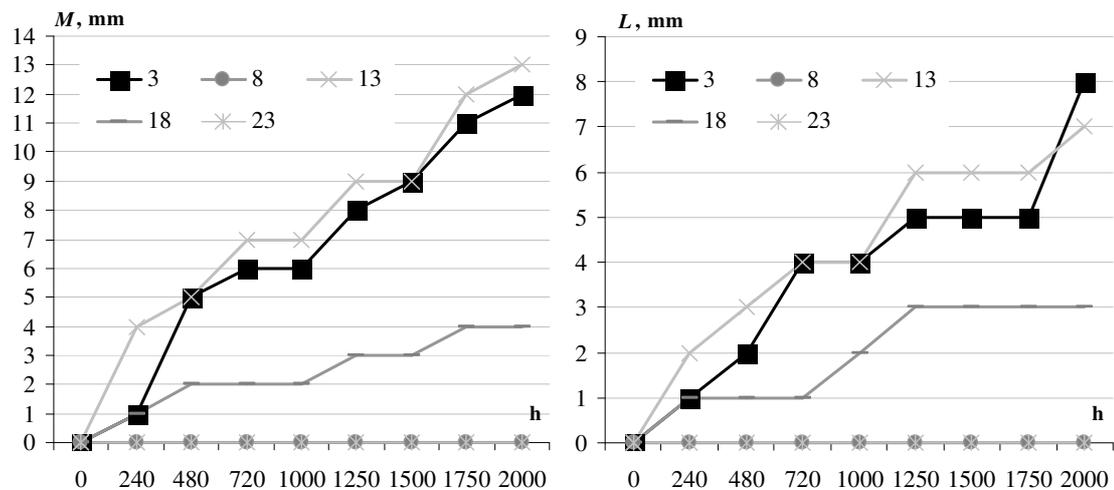
Fig. 2. Spot welding panels characteristics from degree of filiform corrosion - EN ISO 4627-10
