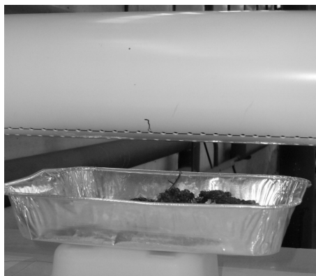
Fig. 1. Forced convective drying of poultry manure by air streams going from tube to surface of plate with manure
