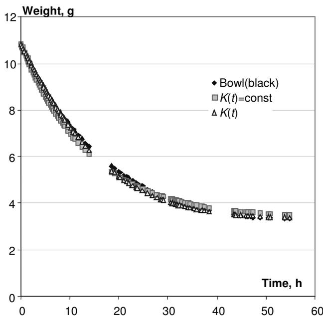
Fig. 4. Linden (*Tilia cordata* L.) flowers' weight change (experimental and theoretical calculated) during drying on a black bowl
