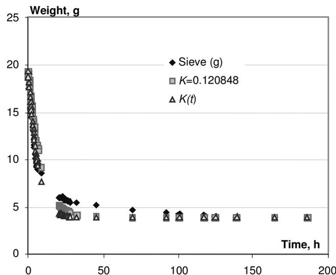
Fig. 6. *Sambucus nigra* L. flower weight change (experimental and theoretical calculated) during drying on a sieve
