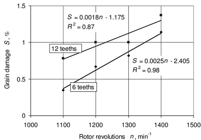
Fig. 5. The influence of rethresher rotor revolutions  $n$  to the grain damage of the rethresher  $S$
