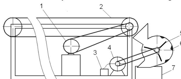
**Fig.1. Schematic overview of the structural parameters and performance indicators of the vane-type rethresher experimental unit:** 1, 4 – electric motors; 2 – belt-conveyor; 3 – power meter; 5 – rotor of the rethresher; 6 – toothed concave; 7 – tailings collection container
