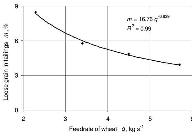
Fig. 3. Influence of wheat feed rate of the combine harvester  $q$  to the loose grain part in the rethresher  $m$
