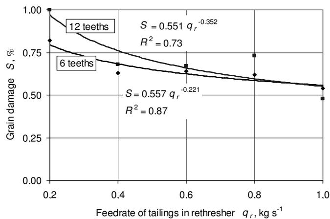
Fig. 6. Influence of tailings feed rate in the rethresher  $q_r$  to grain damage  $S$
