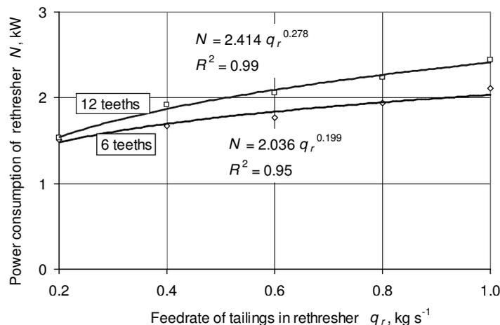
Fig. 8. Influence of tailings feed rate in the rethresher  $q_r$  to the power consumption required for rotation of the rethresher rotor  $N$
