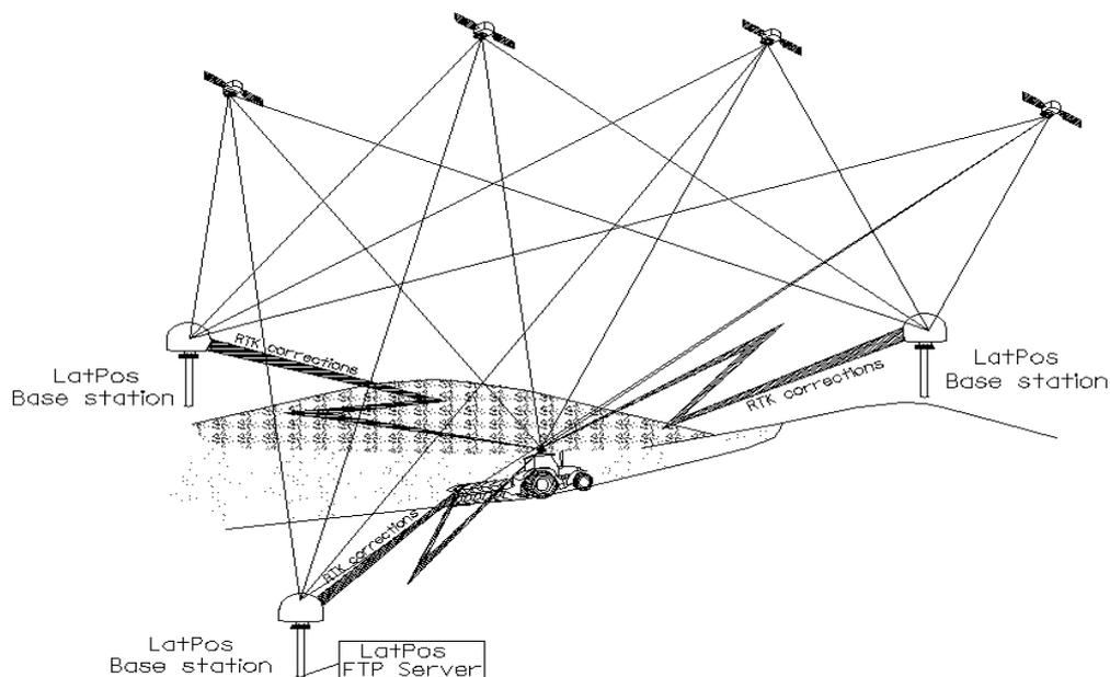
Fig. 2. Precise DGPS data acquisition network system solutions
