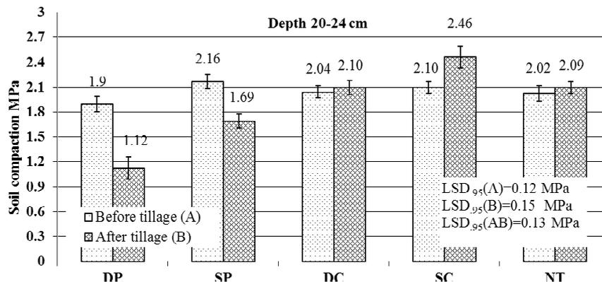
Fig. 3. Soil compaction (in the depth of 20-24cm) before and after autumn soil tillage
