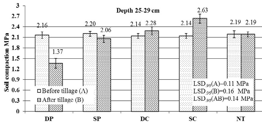
Fig. 4. Soil compaction (in the depth of 25-29 cm) before and after autumn soil tillage
