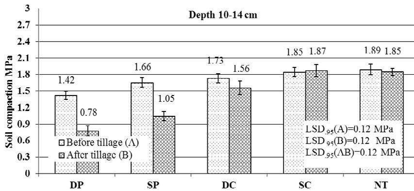
Fig. 2. Soil compaction (in the depth of 10-14 cm) before and after autumn soil tillage
