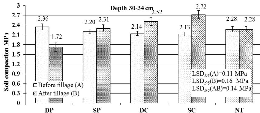
Fig. 5. Soil compaction (in the depth of 30-34 cm) before and after autumn soil tillage
