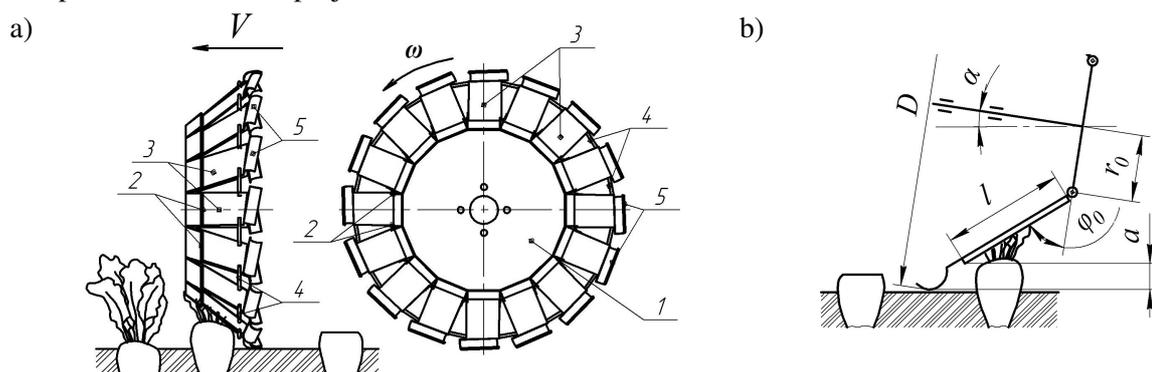
Fig. 1. Operating element for sugar beet topping; a – scheme of operation; b – scheme of design parameters: 1– disk; 2 – joints; 3 – rectilinear part of the operating element; 4 – supports for raising the operating element to a preset height of topping; 5 – cutting part of the operating element
