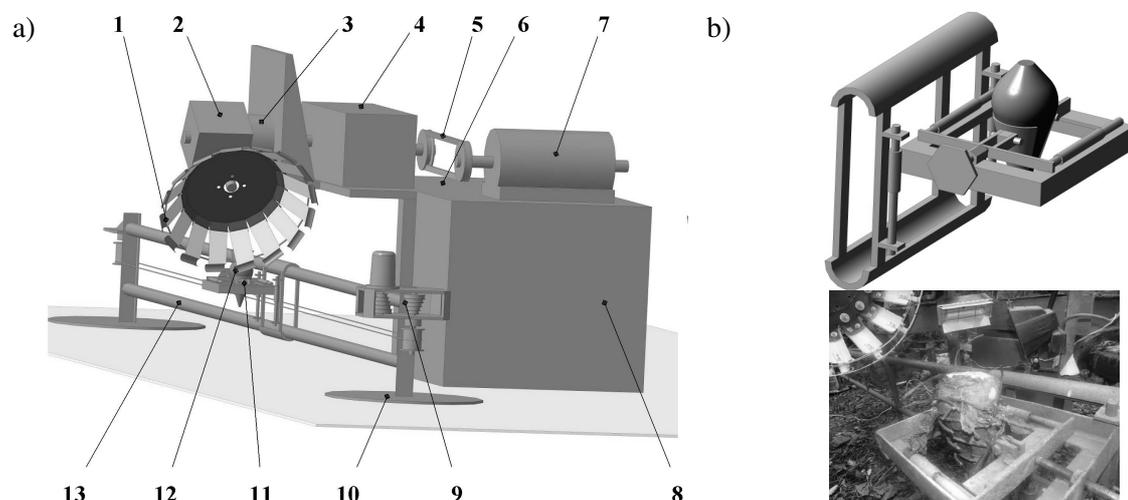
Fig. 2. Scheme of the laboratory equipment for investigation of the top removal process: a – general view; b – frame for fixing the root crop (the photo and 3D model)
