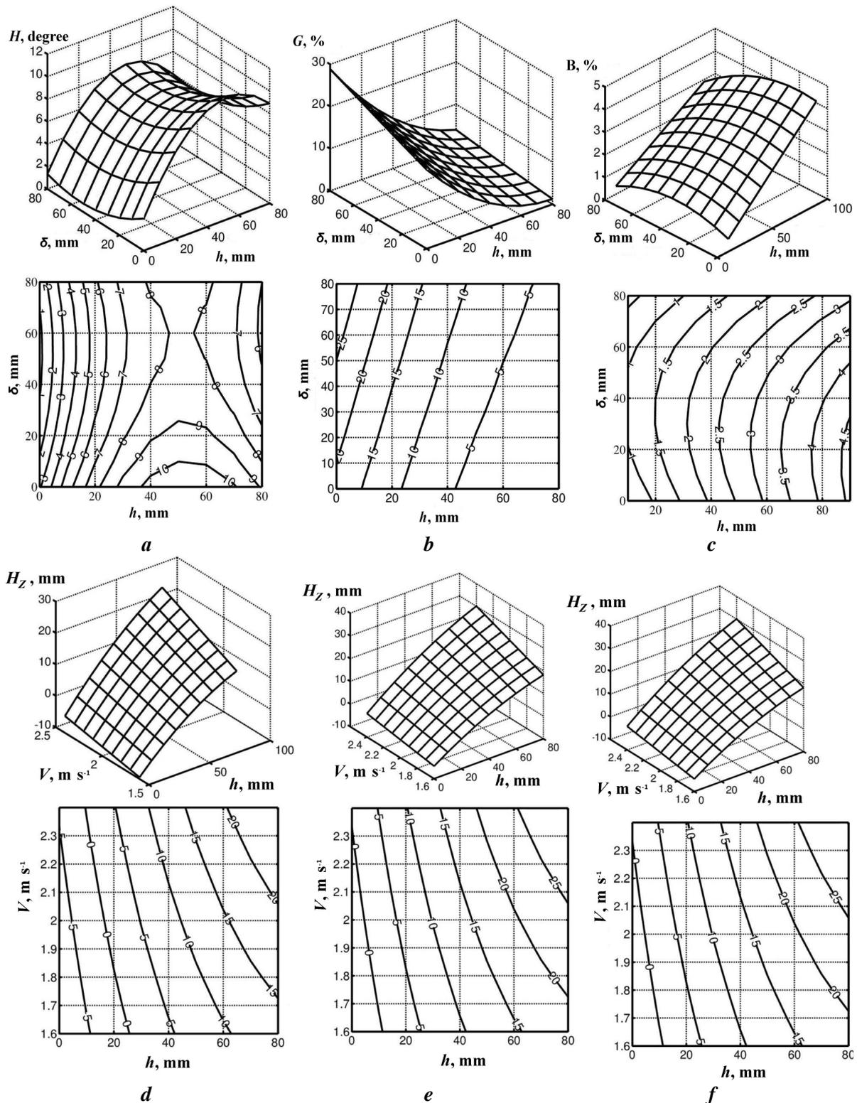
Fig. 3. Dependencies of the quality indicators of the topping process: *a, b, c* – deviation of the shear plane from the horizontal  $H$ , remnants of leaves on the root crops  $G$  and losses of the sugar-bearing mass  $B$ , respectively, from the parameters  $\delta$  and  $h$  at  $a = 25$  mm; *d, e, f* – deviation of the corresponding topping height of the root crop heads  $H_z$  from the parameters  $V$  and  $h$  at  $a = 10, 25, 40$  mm and  $\delta = 40$  mm.
