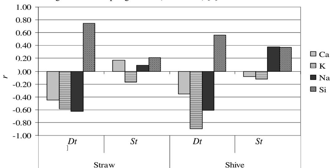
Fig. 1. Hemp ( $n = 15$ ) correlations between ash melting temperature and chemical content:
