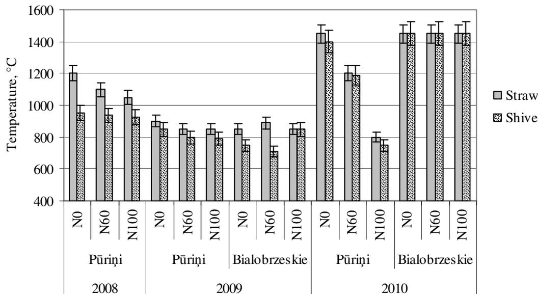
Fig. 3. Ash melting deformation temperature of hemp in Latvia depending on experiment year, variety and N fertiliser norm
