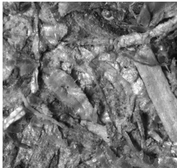
Fig. 2. Macrostructure at the center of the bio-briquette after the third stage of pressing (silvery inclusion – binding lignin)
