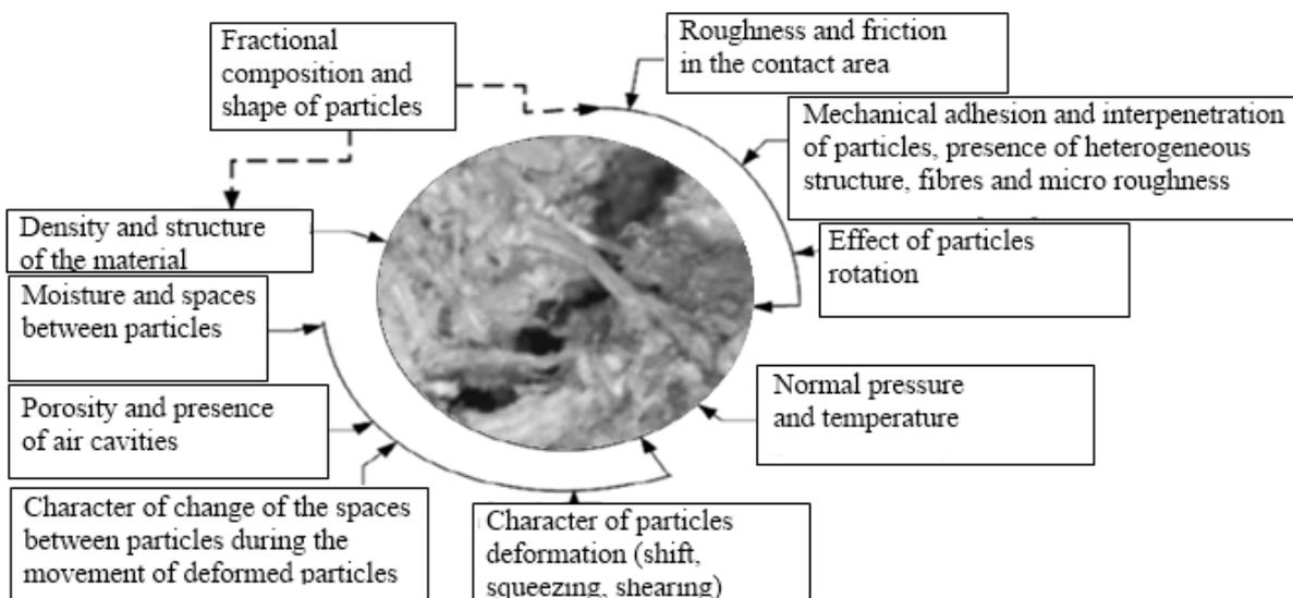
Fig. 4. Factors influencing the pressing process of the biomass composition mixture
