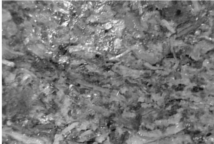
Fig. 3. Typical macrostructure of lateral surface of the bio-briquette
