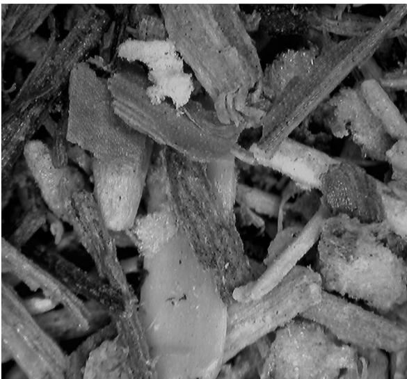
Fig. 1. Original mixture of crushed vine pruning and corn straw
