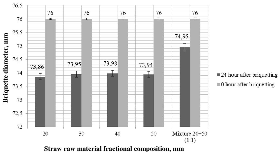
Fig. 1. Changes of briquette diameter values
