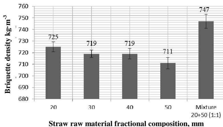
Fig. 2. Density of briquettes from straw chaff with different fractional composition
