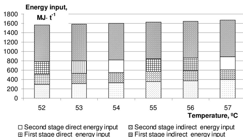
Fig. 2. Total energy input at biogas plant
