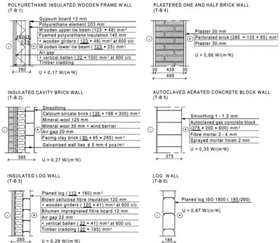
Fig. 2. Details of the external wall structures of the test buildings
