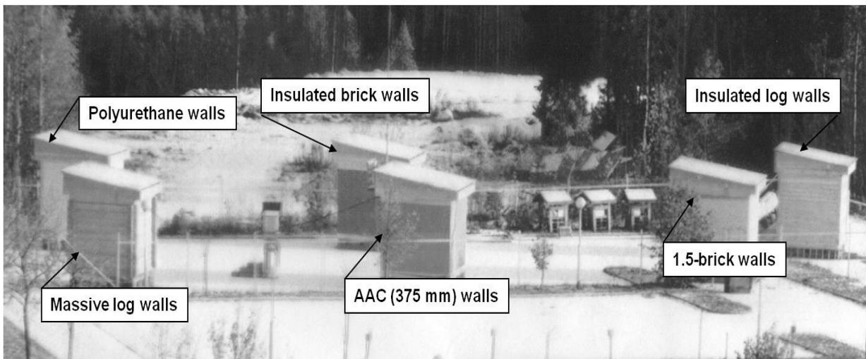
Fig. 1. Test buildings at RTEK/TUT
