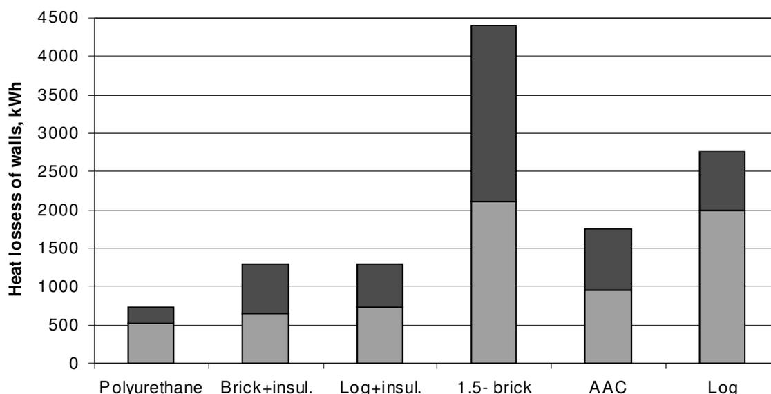
Fig. 3. Measured (light grey bars) and calculated (light grey + dark grey bars) heat losses of the walls of the test buildings at TUT from Sept. 1998 to May 1999 [9]
