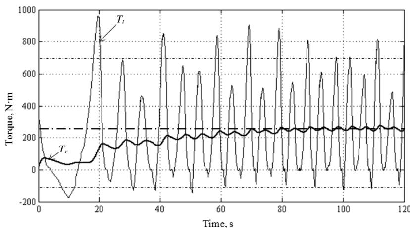
Fig. 6. Wind turbine torque simulation with variable wind speed
