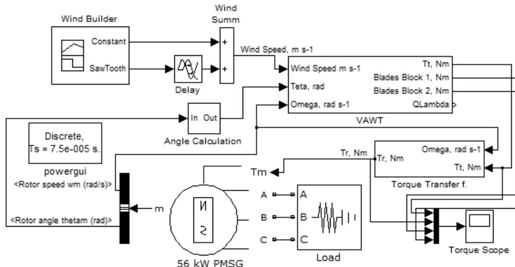
Fig. 3. Wind turbine virtual model in MATLAB SIMULINK
