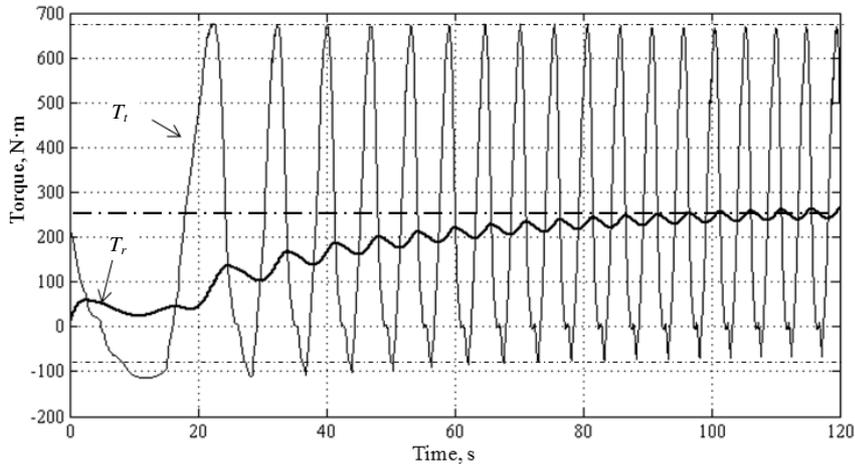
Fig. 5. Wind turbine torque simulation with constant wind speed  $4 \text{ m}\cdot\text{s}^{-1}$
