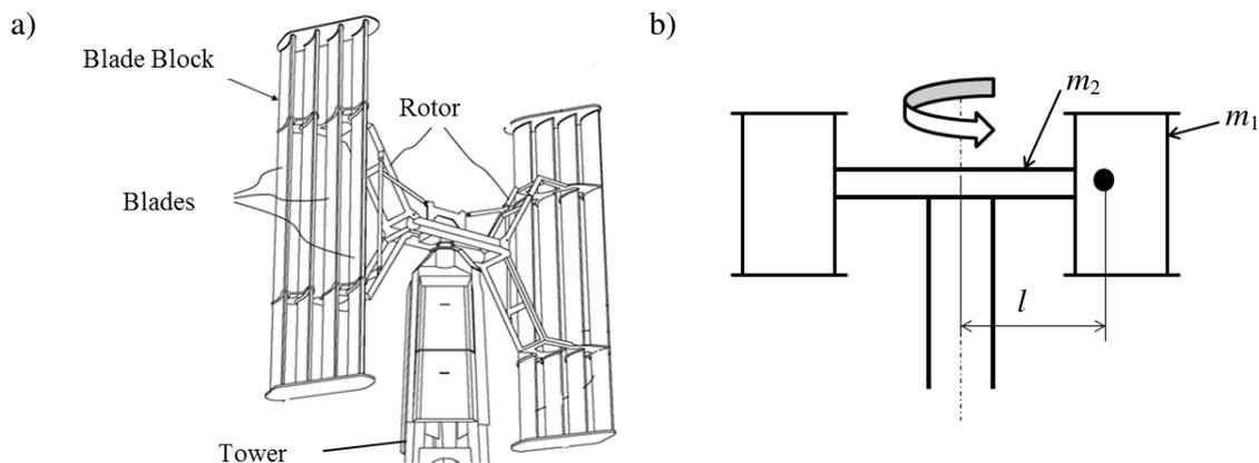
Fig. 2. Wind turbine mechanical design according to the patent: a – full structure; b – simplified structure for calculation of the moment of inertia ( $m_1$  – blade block mass, kg;  $m_2$  – rotor mass, kg;  $l$  – radius of the mass centre)
