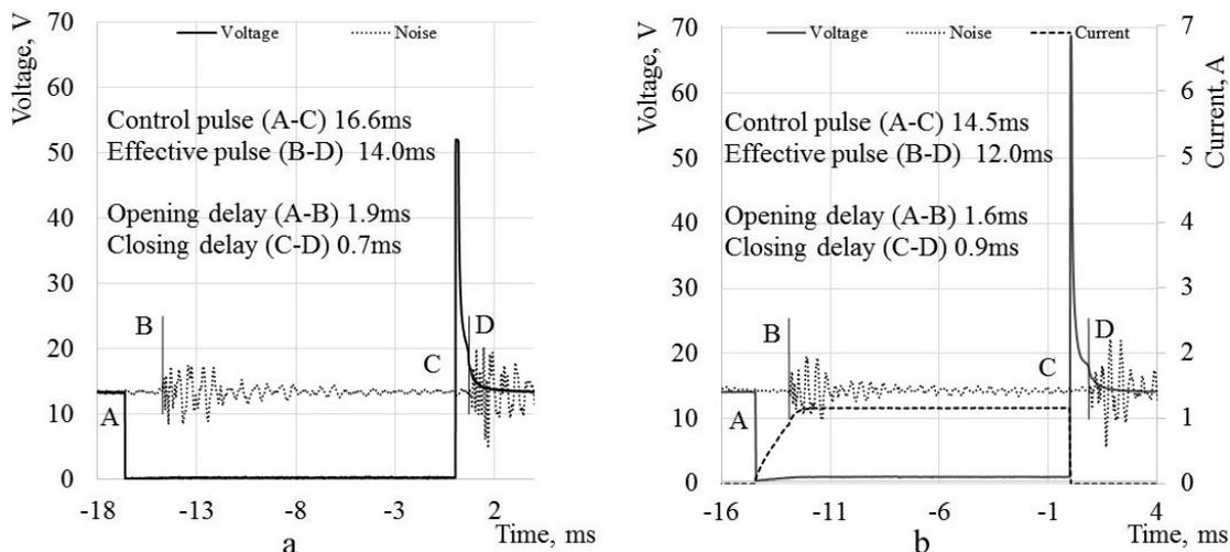
Fig. 2. Characteristic curves of the injector control: a – Renault Twingo; b – Volkswagen Passat
