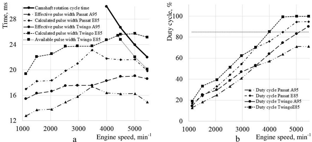
Fig. 3. **Operational curves:** a – injector pulse time; b – injector duty cycle
