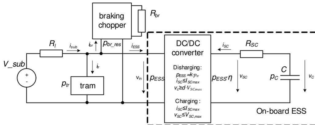
Fig. 1. Block diagram of electric transport feeding system and tram equipped with ESS
