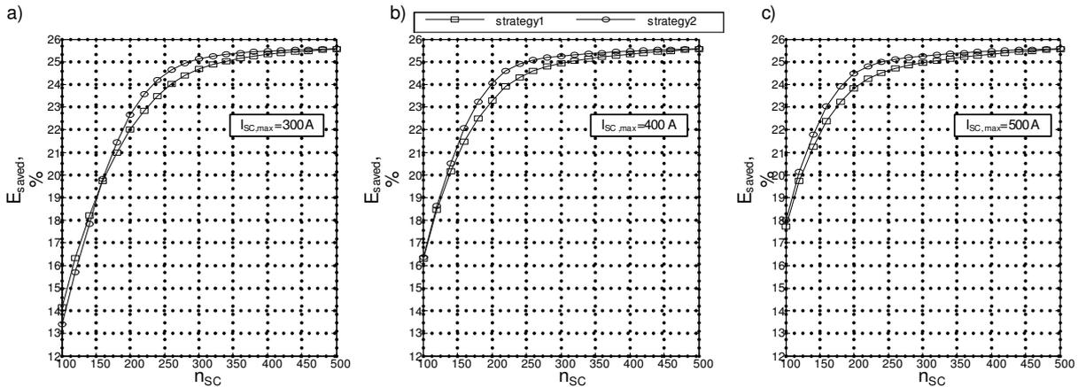
Fig. 5. Comparison of ESS efficiency with different control strategies
