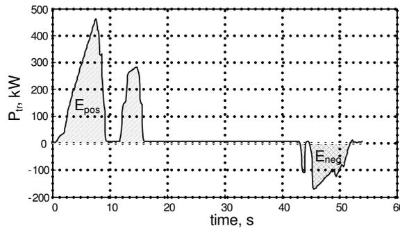
Fig. 3. Tram power diagram between two stops
