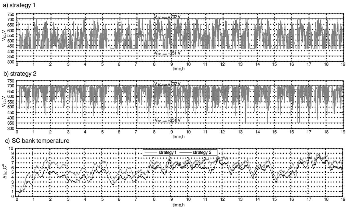
Fig. 6. SC bank voltage and temperature diagrams
