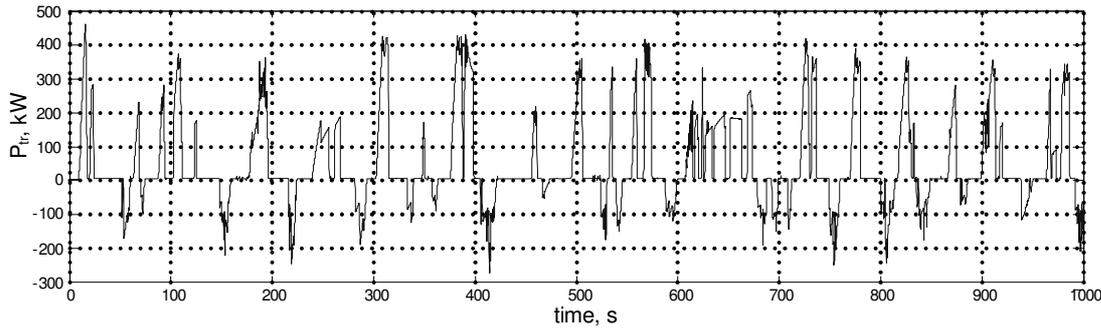
Fig. 2. Experimentally measured tram power diagram
