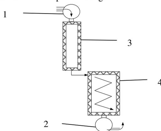
Fig. 1. A principal general view of the experimental equipment: 1 – the sealing/dosing units; 2 – the dosing units for the water adsorbent granules, 3 – the bioethanol dehydration column; 3 – the regenerator for the water adsorbent granules
