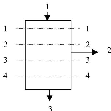
Fig. 2. Scheme of experimental facility's water adsorption granule regenerator: 1 – inlet; 2 – vapour extraction; 3 – discharge
