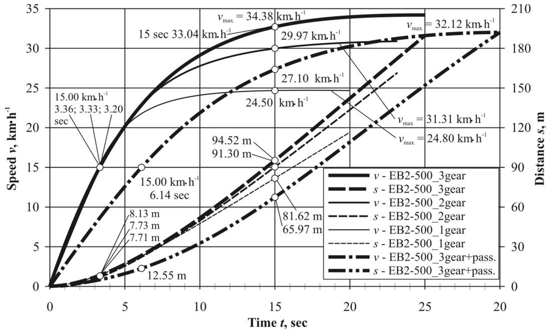
Fig. 6. Acceleration characteristics testing EB2-500 electric bicycle
