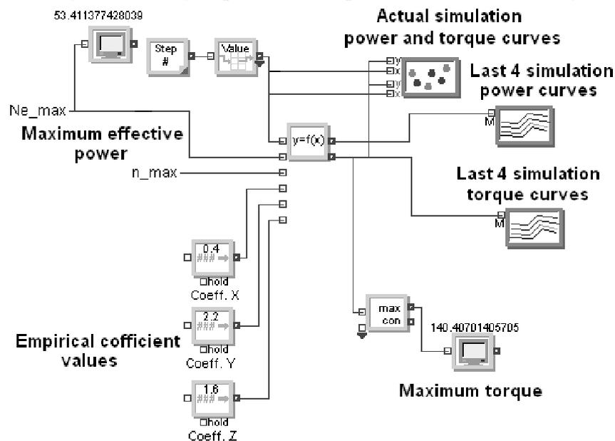
Fig. 6. Model blocks for constructing of diesel engine power and torque curves
