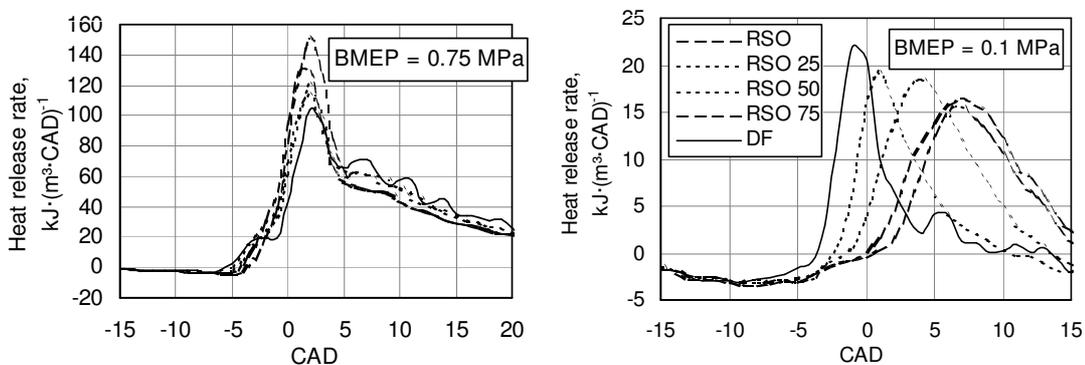
Fig. 3. Amount of RSO in blend influence on heat release rate ( $n = 1400 \text{ min}^{-1}$ )
