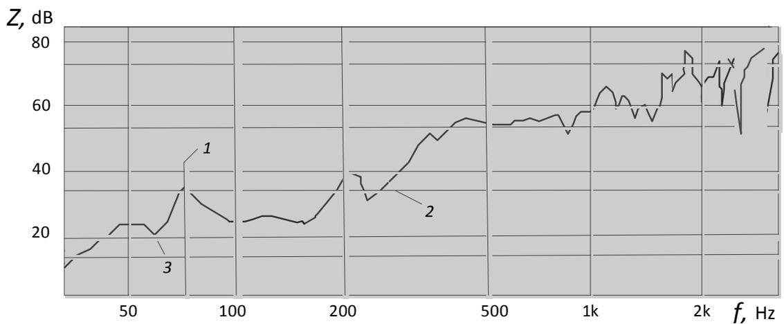
Fig. 5. Transient mechanical impedance frequency spectrum: 1 – without oil; 2 – with oil type 10W40; 3 – with oil type 80W90
