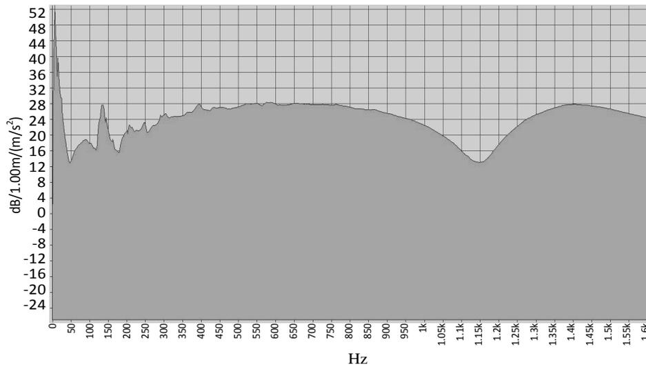
Fig. 4. Frequency response function (FFT), with oil type 80W90
