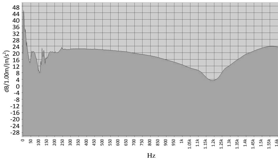
Fig. 3. Frequency response function (FFT), with oil type 10W40
