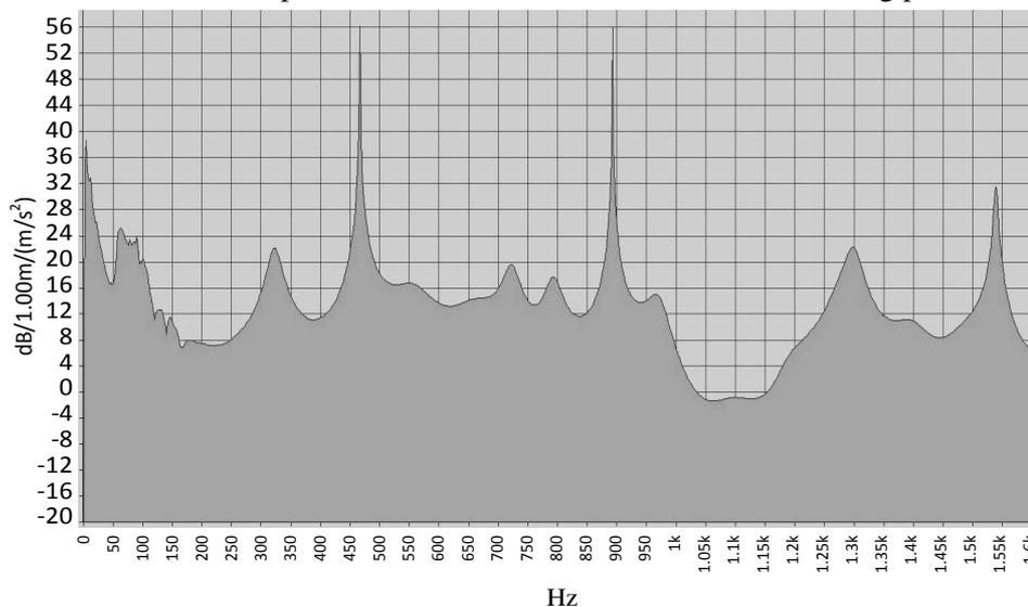
**Fig. 2. Frequency response function (FFT), excitation without oil**
