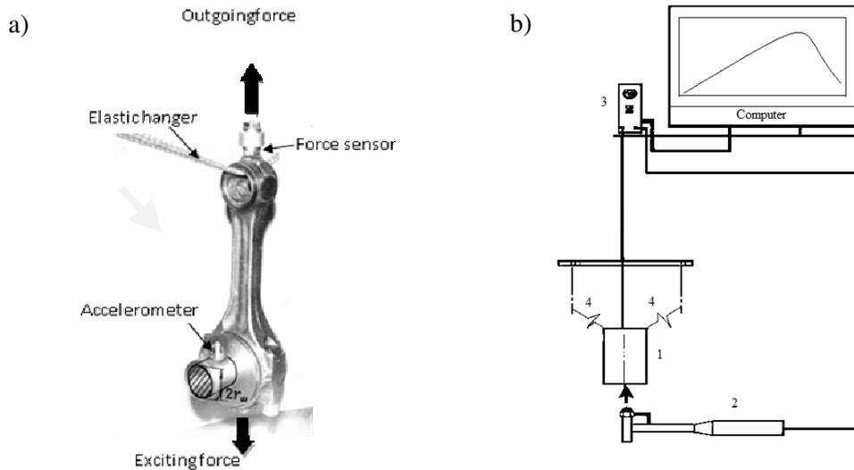
**Fig. 1. Accelerometer and impact force locations (a) and experimental set-up for measurement of mechanical impedance (b):** 1 – piston-rod; 2 – impact hammer; 3 – data acquisition; 4 – elastic construction hangers
