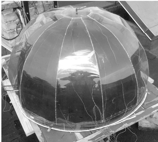
**Fig.1. Semi-spherical solar collector [3]**
