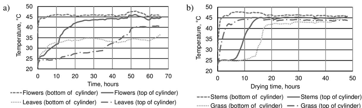
Fig. 3. Changes of drying agent temperature: a – in a mound of dried flowers and leaves; b – in a mound of dried stems and grass
