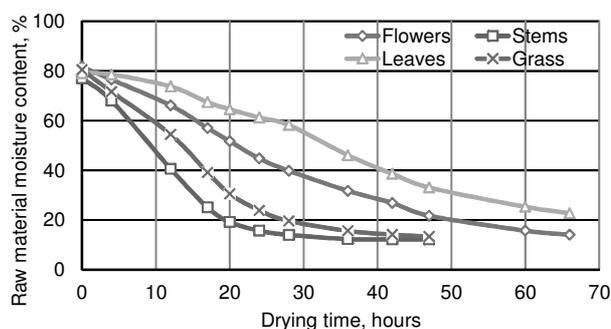
Fig. 2. Dynamics of herbal raw material (*Echinacea purpurea* L. Moench) drying in a thick still mound
