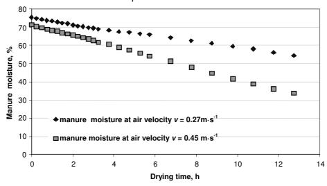
Fig. 5. Manure moisture changes during the drying process by convection with air speeds at top 0.27 m·s<sup>-1</sup> and 0.45 m·s<sup>-1</sup>
