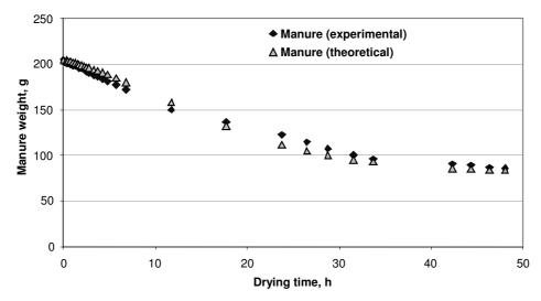
Fig. 4. Manure weight changes during the drying process by convection with air speed at top 0.27 m·s<sup>-1</sup>
