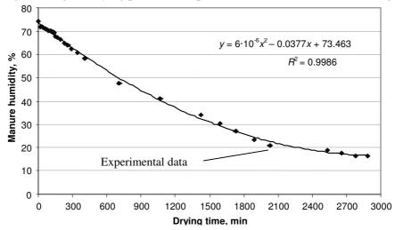
Fig. 3. Manure humidity changes by convection with air speed at top 0.27 m·s<sup>-1</sup>
