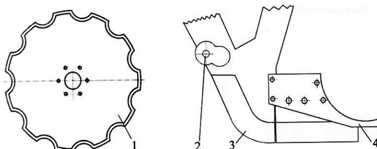
Fig. 1. **Complex sowing couler parts:** 1 – disc knife with notched blades; 2 – mounting place of the disc knife; 3 – hob coultter with extended hob; 4 – mount of sowing apparatus
