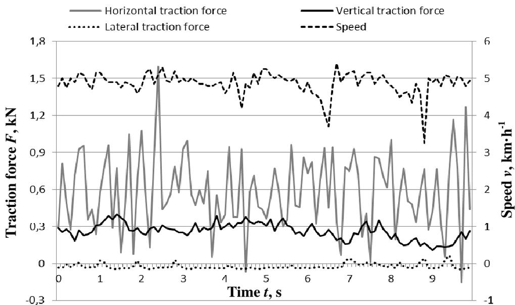
Fig. 3. Traction forces of hob coultter in the soil of 0.493 MPa hardness
