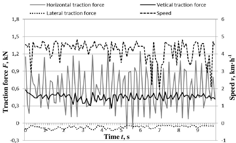
Fig. 2. Traction forces of hob coultter in the soil of 0.044 MPa hardness
