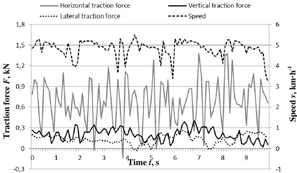
Fig. 4. Traction forces of hob coulters in the soil of 0.827 MPa hardness
