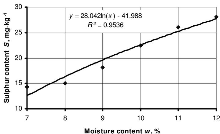
Fig. 2. Influence of moisture content  $w$  of pressing rapeseed on sulphur content  $S$  when pressing temperature  $t$  was 50 °C
