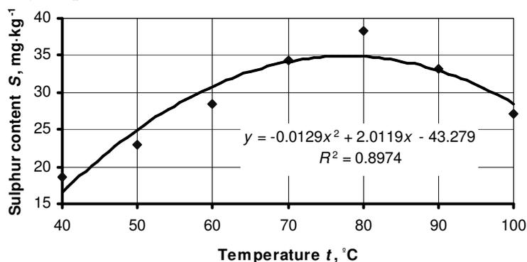
Fig. 1. Influence of pressing temperature  $t$  on sulphur content  $S$
