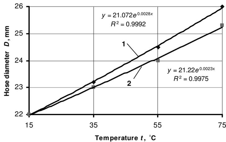
Fig. 3. Changes of rubber hose diameter in oil of: 1 – rapeseed; 2 – linseed
