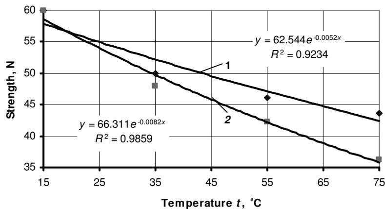
Fig. 4. Change of rubber hose surface strength in oil of: 1 – rapeseed; 2 – linseed
