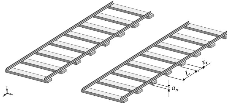
Fig. 4. Scheme of artificial roughness road
