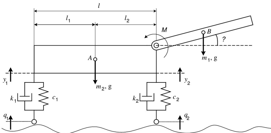
Fig. 1. Mechanical model of tractor aggregate with mounted implement
