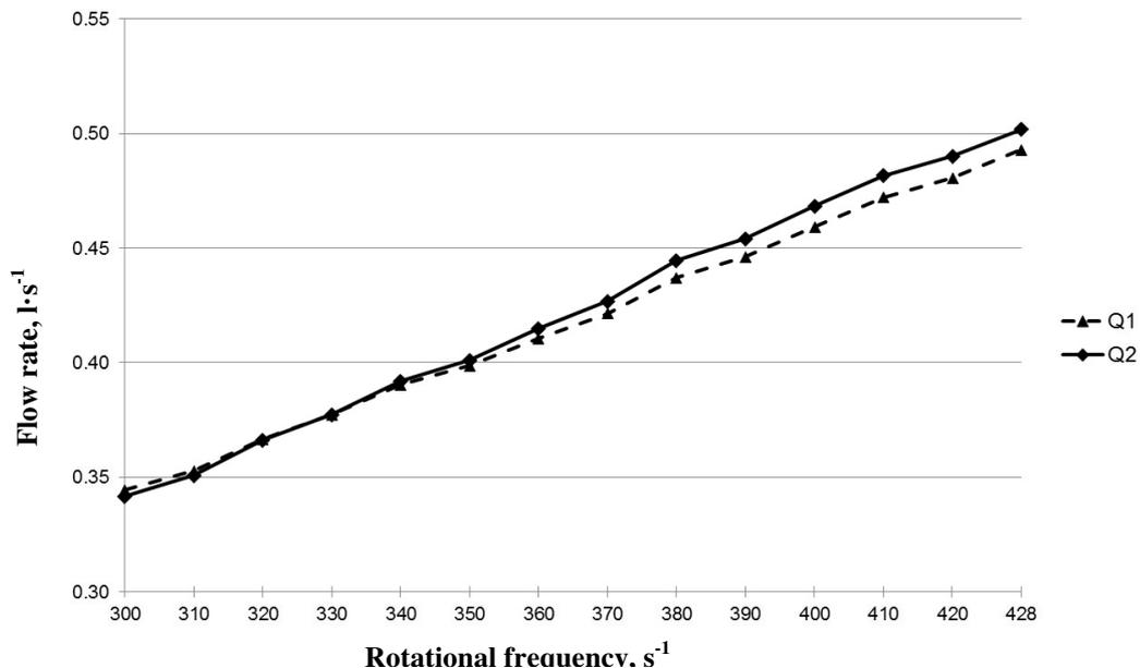
Fig. 6. Details of graph depicting dependency of hydraulic oil flow on cutting disc rotational frequency: Q1 – flow of hydraulic oil in pressure line; Q2 – flow of hydraulic oil in drain line
