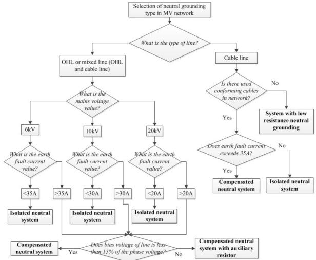
Fig. 4. Selection of neutral grounding type in MV network
