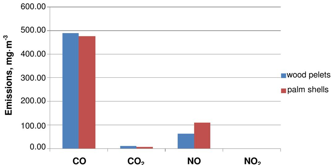
Fig. 3. Comparison of emissions from combustion of wood pellets and palm shells
