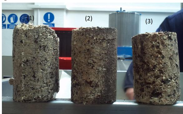
**Fig. 2. Samples of briquettes made of mixture of palm shells and wood shavings in ratio 1:1 by weight: 1 – palm shells ground to 3.8 mm; 2 – palm shells ground to 8 mm; 3 – not ground palm shells**
