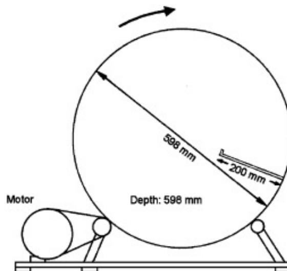
Fig. 1 Briquette durability tester
