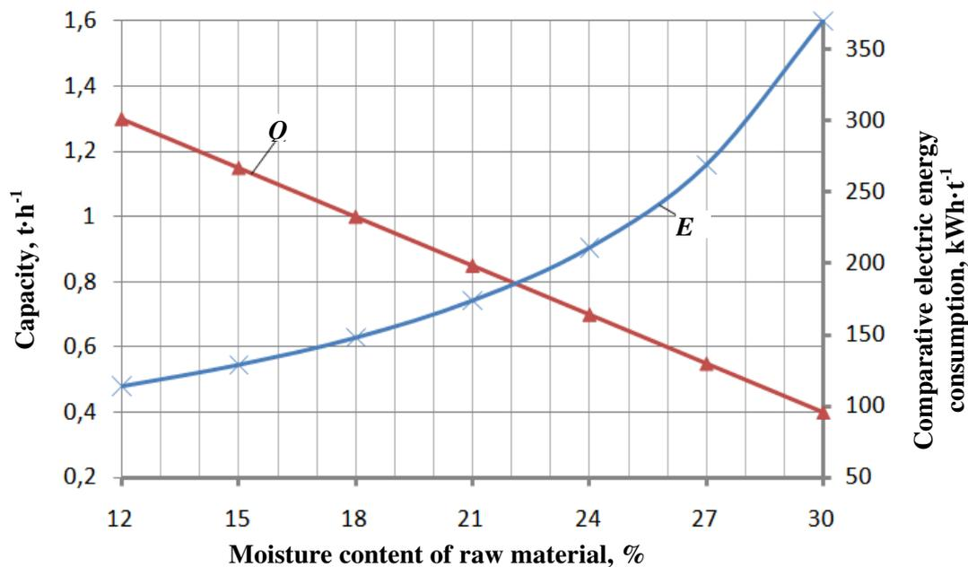
Fig. 3. Variation of the technological line capacity and energy consumption:  $Q$  – capacity of technological line subject to moisture content of raw material,  $t \cdot h^{-1}$ ,  $E$  – variation of comparative electric energy consumption subject to moisture content of raw material,  $kWh \cdot t^{-1}$
