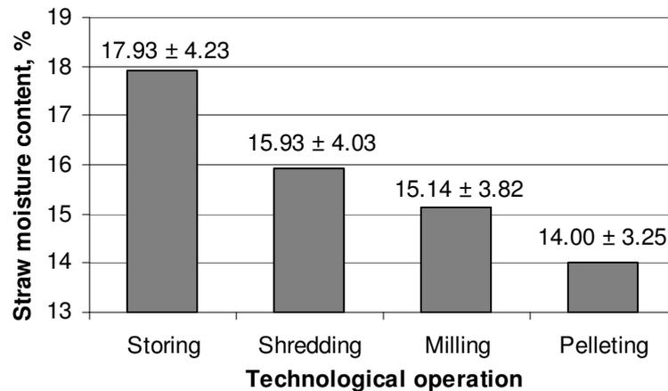
Fig. 2. Variations of straw moisture content in the technological line
