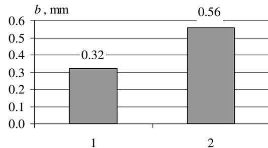
Fig. 13. The deterioration of chain plates  $\Delta b$  (experiment bench No. 2):
