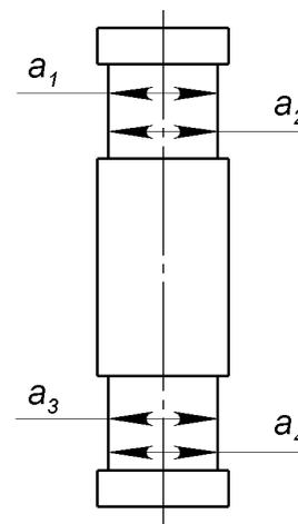
Fig. 6. Roller of a sliding friction hinge:  $a$  – measurements of the deterioration of the roller effective surfaces
