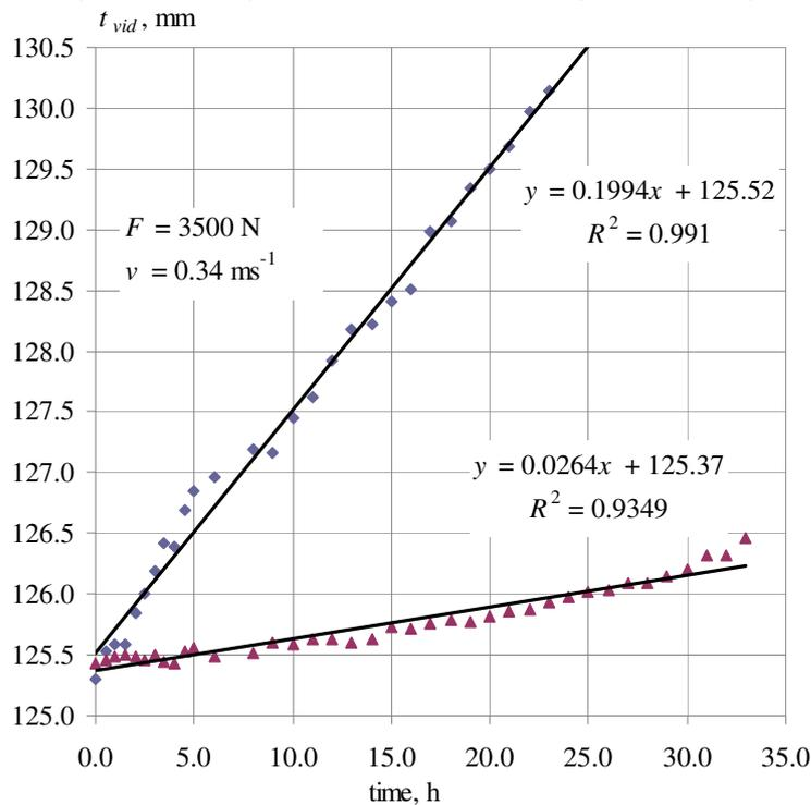
Fig. 8. The average chain pitch angle  $t_{vid}$  (experiment bench No. 1):
