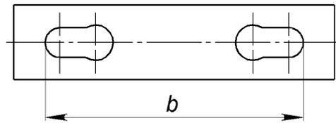
Fig. 4. Plate of the sliding friction hinge chain:  $b$  – gap between the straight effective surfaces of the plate
