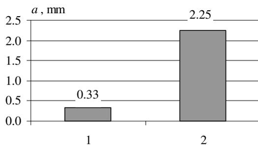
Fig. 12. The deterioration of chain plates  $\Delta a$  (experiment bench No. 2):
