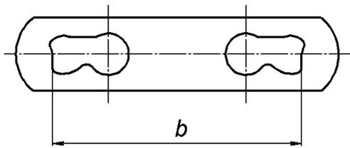
Fig. 3. Plate of the rolling friction hinge chain:  $b$  – gap between the straight effective surfaces of the plate
