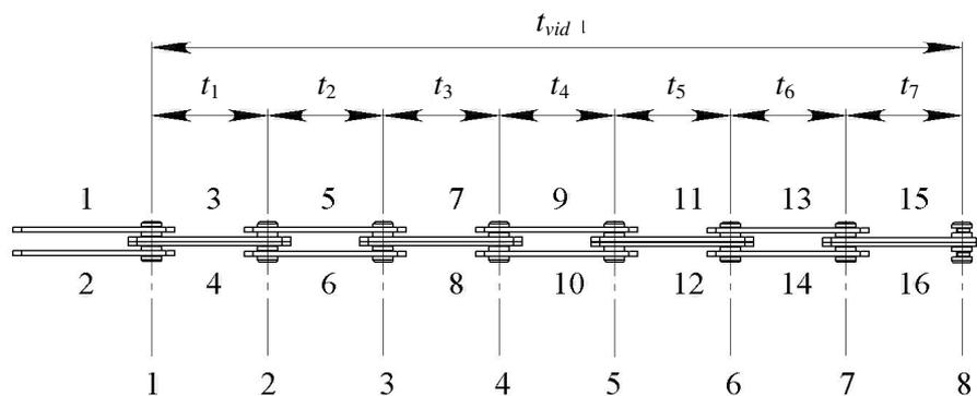
Fig. 7. Layout of measuring the chain link pitch: applicable to the links 1 and 2 of both rolling friction hinges and sliding friction hinges
