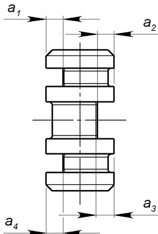
Fig. 5. Roller of a rolling friction hinge:  $a$  – measurements of the deterioration of the roller effective surfaces
