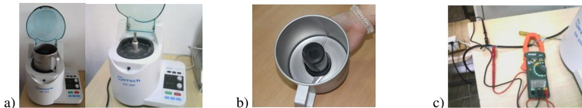
Fig. 1. Laboratory mill Grindomix GM-200 (a); stainless steel tray and knives (b); power clamp meter EXTECH model 380976 (c)
