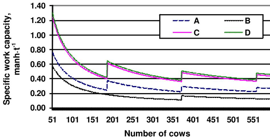
Fig. 1. Specific consumption of work for preparation and distribution of animal feed mix,  $\text{manh}\cdot\text{t}^{-1}$ , depending on the number of cows and technological solution
