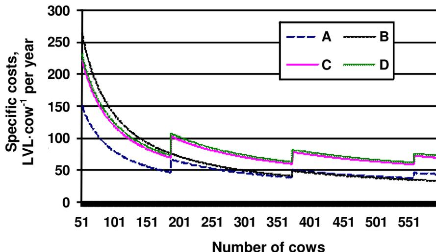
Fig. 2. Animal feed preparation and distribution specific costs,  $\text{LVL}\cdot\text{cow}^{-1}$  per year, depending on the number of cows on the farm and the technological solution used
