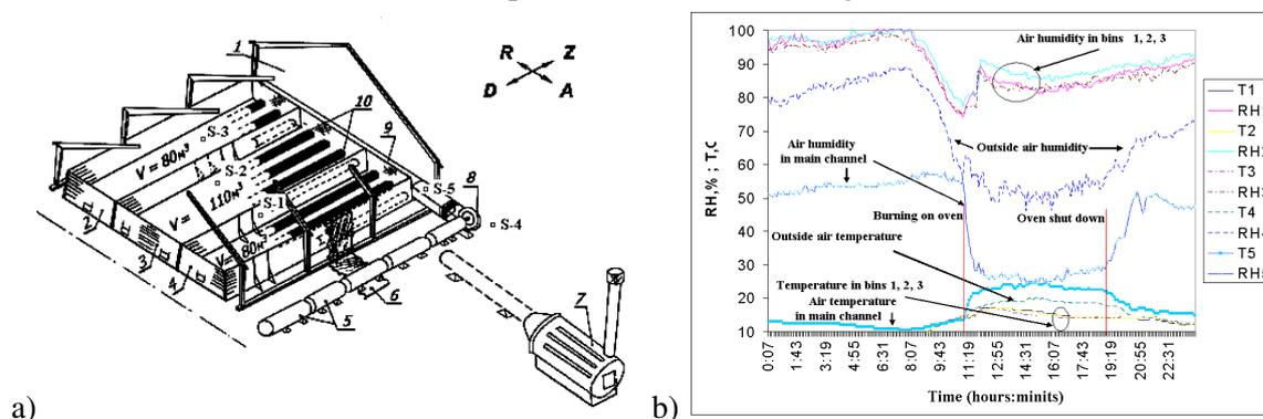
Fig. 4. Scheme of ecological grain drier-storage plant having ventilated bins provided with sensors (a) and single-day monitoring results of the grain drying process as an example (b): 1 – barn; 2, 3, 4 – ventilated grain drying-storage bins; 5 – air collectors; 6 – solar energy absorption film; 7 – heat generator (furnace) 40 kW; 8 – radial fan HL 15; 9 – main air channel; 10 – operating channels; S-1, S-2, S-3, S-4, S-5, S-6 – sensors DS1923
