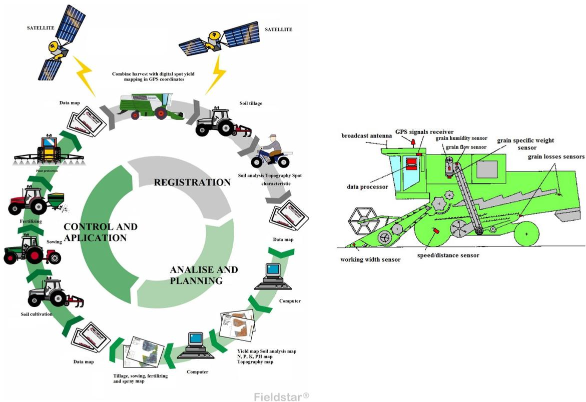
Fig. 1. Cycle of information and measures to application GPS technologies in the Precision Agriculture. Equipment of the combine grain harvester for the determination and mapping spot yields in GPS coordinates
