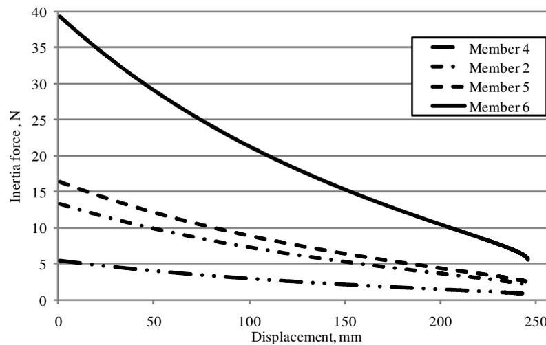
Fig. 6. Inertia force of mechanism members
