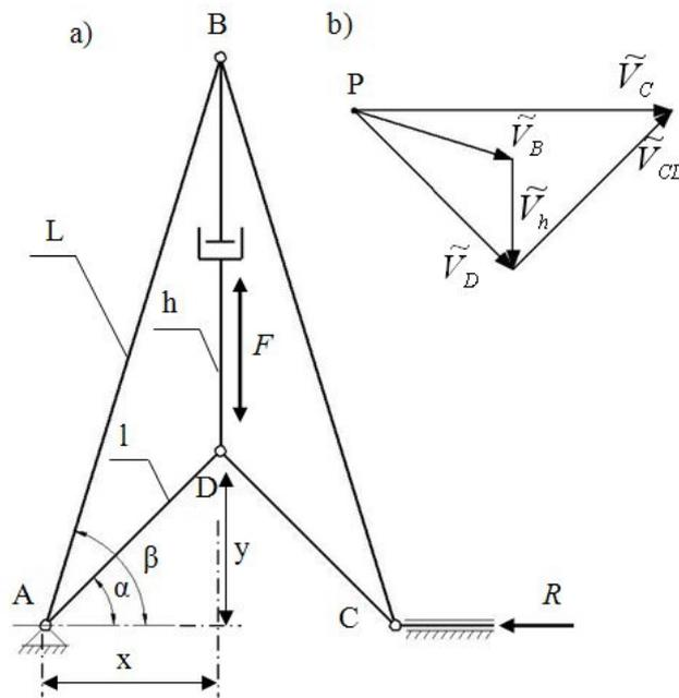
Fig. 3. **Structural scheme:** a – rhomboid mechanism; b – velocity vectors; L, l – length of mechanism members; h – length of hydraulic cylinder
