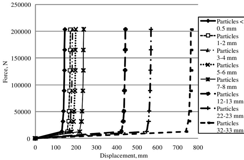
Fig. 4. Force – displacement characteristics of compacting
