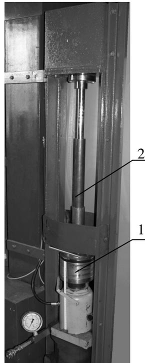
Fig. 1. **Hydraulic press:** 1 – press cylinder; 2 – closed die
