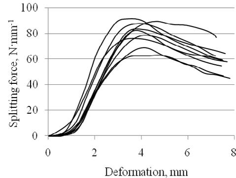
Fig. 4. **Force – deformation diagram for not flattened reed stalks, 300 mm length**
