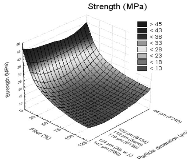
Fig. 4. Strength of multipurpose specimens
