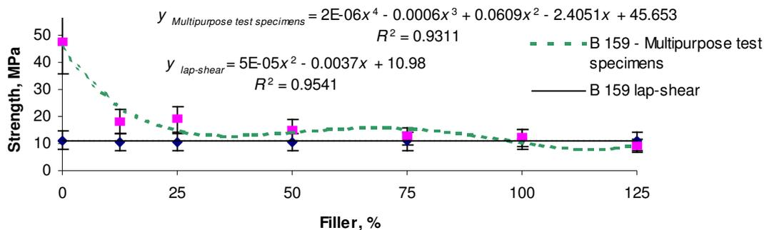
Fig. 5. Graphical representation of the lap-shear strength and multipurpose specimen strength using the filler B 159
