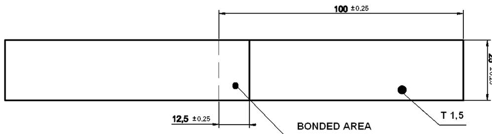
Fig. 1. Shape and dimensions of specimen – tensile shear strength
