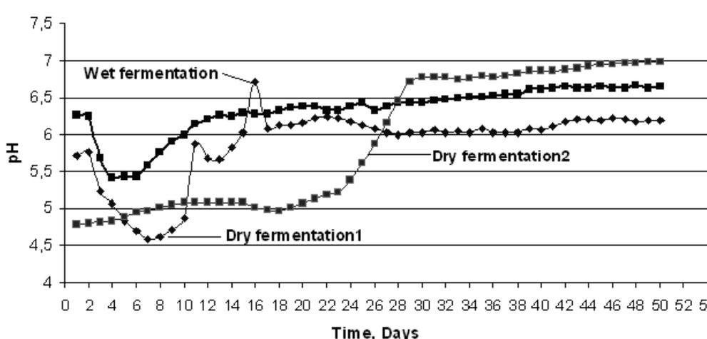
Fig. 3. Variable pH, dry and wet fermentation
