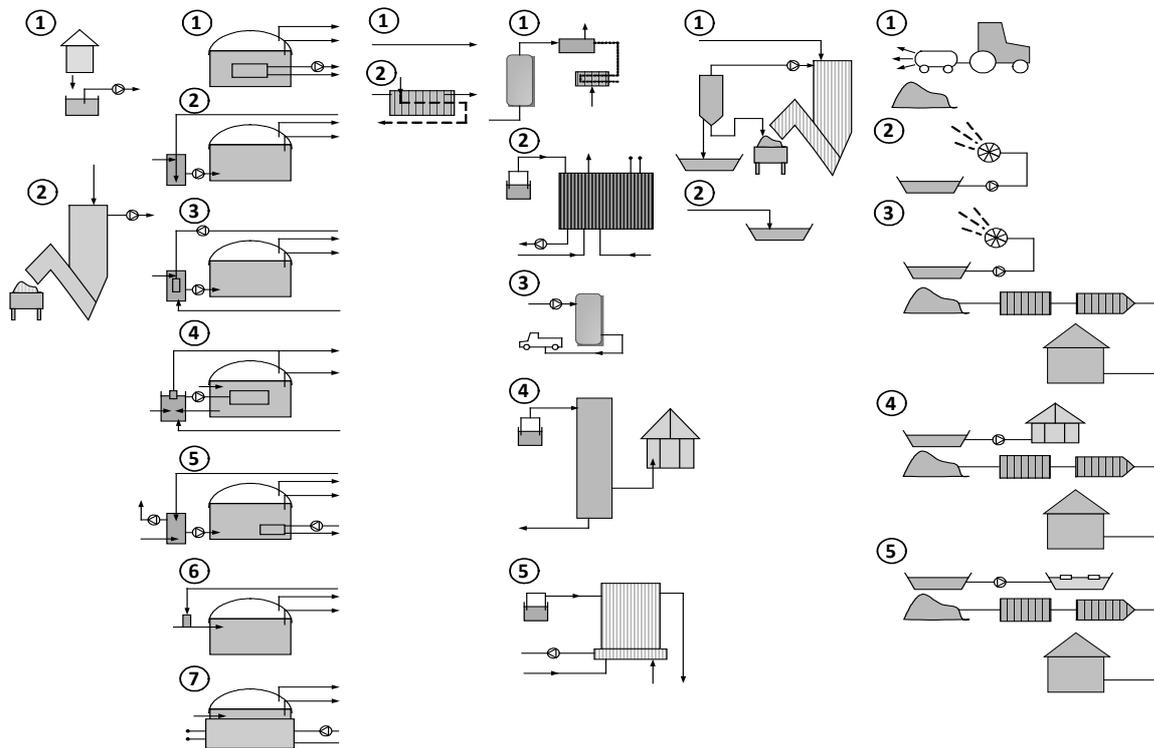
Fig. 2. Biogas technology elements for design of biogas plant
