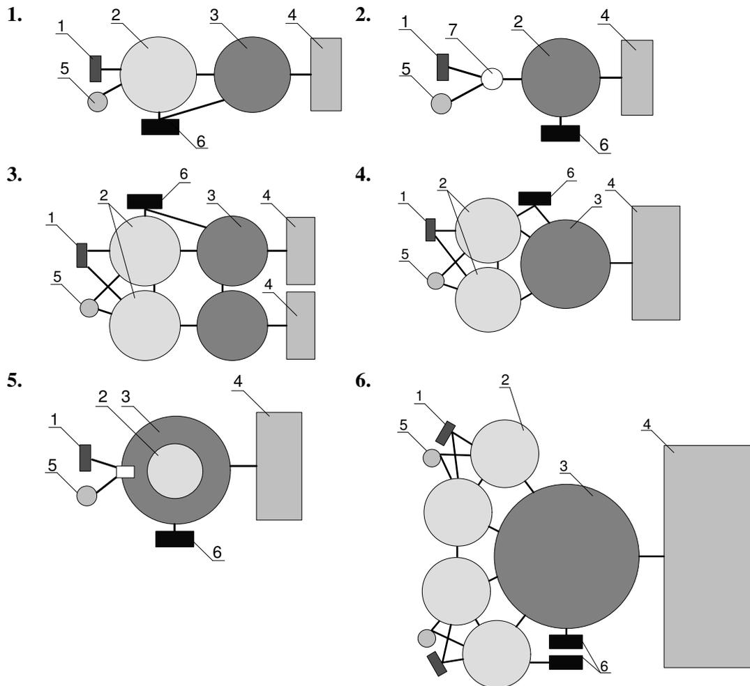
Fig. 1. **Principal technological schemes for Latvia biogas plants:** 1 – tank for dry biomass; 2 – fermenter; 3 – postfermenter; 4 – digestate storage; 5 – wet biomass tank; 6 – CHP unit; 7 – tank for homogenisation
