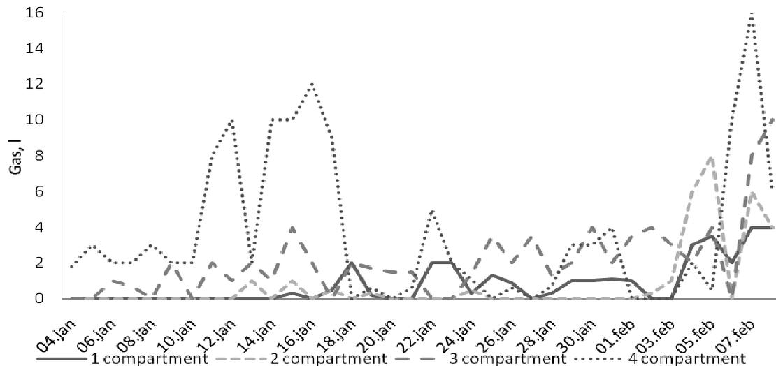
Fig. 5. Preliminary results from four stage digester for anaerobic treatment of biomass: the yield of gas from compartments
