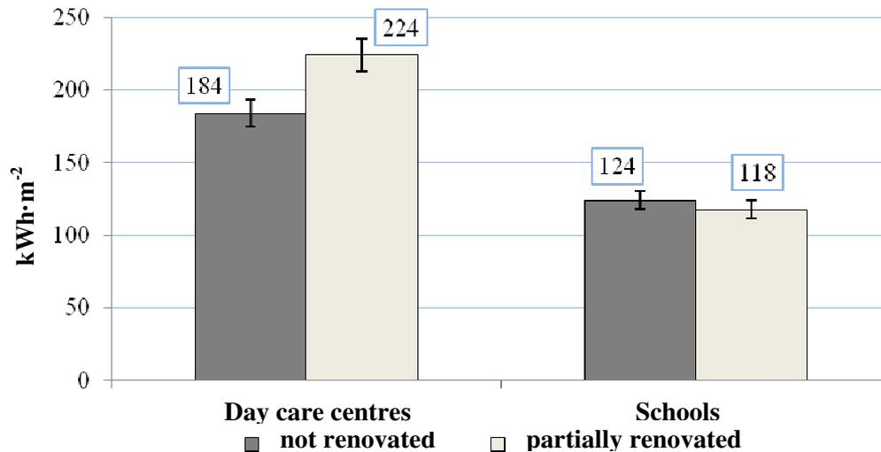
Fig. 2. Average heat energy consumption per annum to one square metre in not renovated buildings and in partially renovated buildings with error bars with 5 % value
