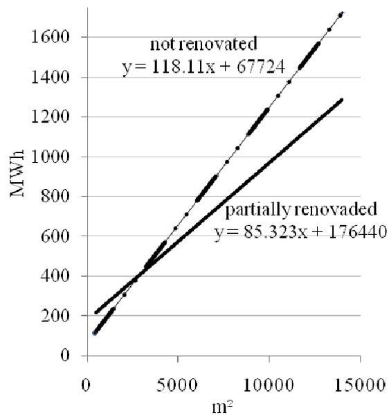
Fig. 8. **Regression lines of the schools from not renovated buildings and partially renovated:** total 158units (not renovated -56 units; partially renovated – 102 units)
