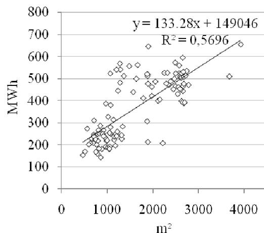
Fig. 4. Partially renovated day-care centre: Total heat energy consumption (MWh) per annum buildings correlation with buildings floor area (m<sup>2</sup>)
