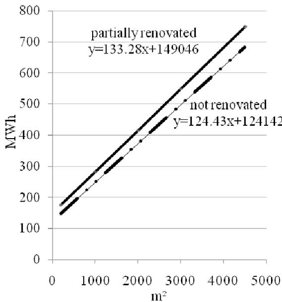
Fig. 7. **Regression lines of the day-care centres from not renovated buildings and partially renovated:** total 143 units (not renovated -32 units; partially renovated – 111 units)
