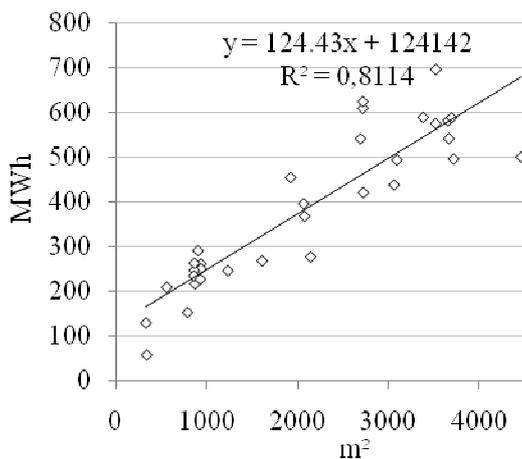
Fig. 3. Not renovated day-care centre buildings: total heat energy consumption (MWh) per annum buildings correlation with buildings floor area (m<sup>2</sup>)
