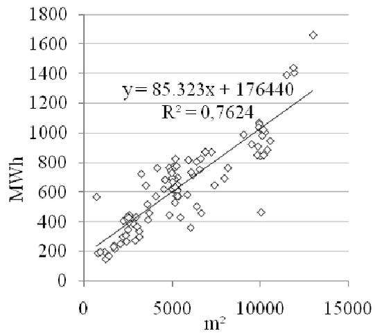
Fig. 6. **Partially renovated school buildings:** total heat energy consumption (kWh) per annum correlation with buildings floor area (m²)
