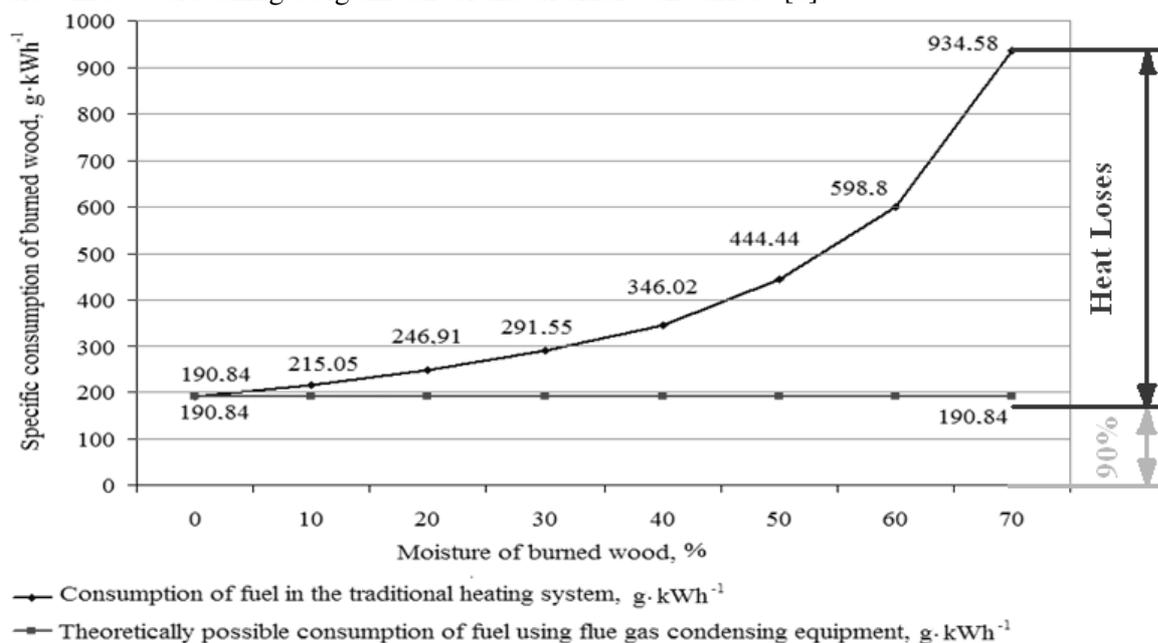
Fig. 3. Dependence of heat energy losses from wood fuel moisture [2; 3]
