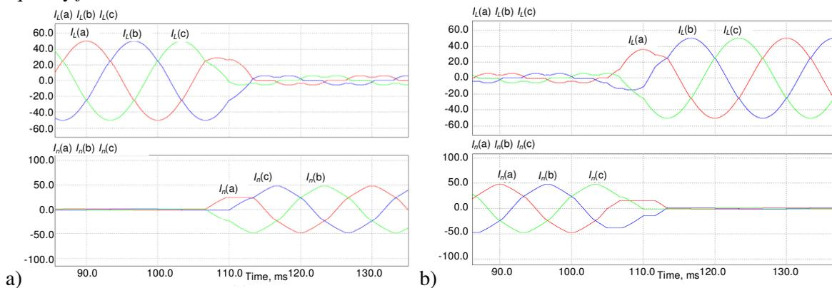
Fig. 3. Reactor current and network current at different reactive powers of reactors during switching at 105 ms: a – from  $Q_L=23$  kVAr to  $Q_L=2.6$  kVAr; b – from  $Q_L=2.6$  kVAr to  $Q_L=23$  kVAr
