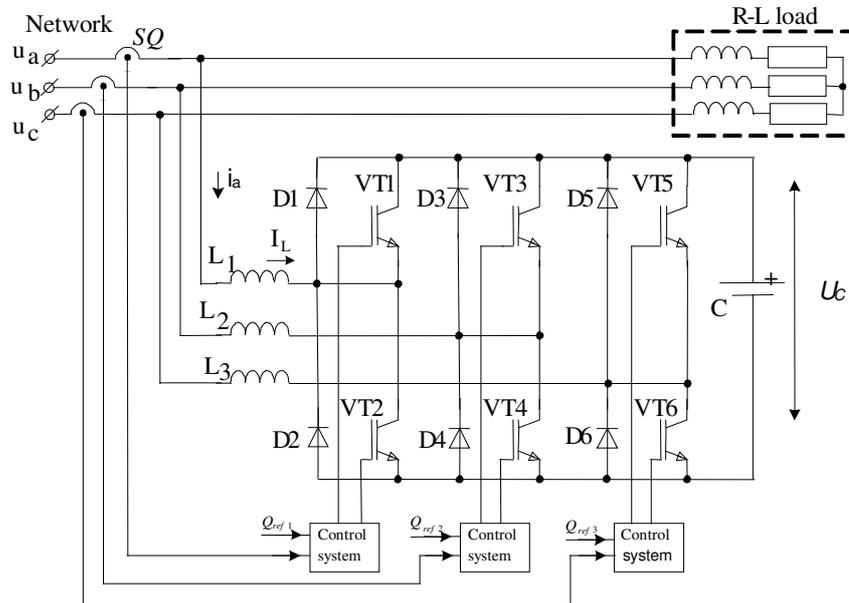
Fig. 2. Generalized power and control circuit of transistorized compensator
