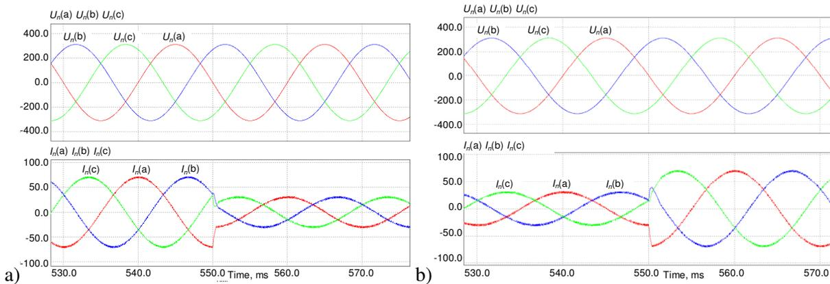
**Fig. 4. Reaction of network voltage and network current before and after changes of the control system reference value: a – from  $Q_{ref}=32.5$  kVAr to  $Q_{ref}=12$  kVAr; b – from  $Q_{ref}=12$  kVAr to  $Q_{ref}=32.5$  kVAr**
