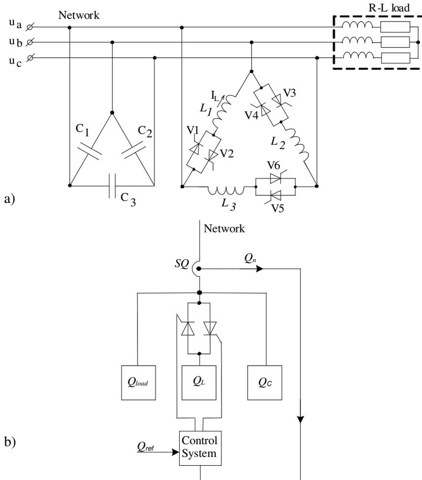
Fig. 1. Generalized flexible reactive power compensation system with thyristor regulated reactors: a – scheme; b – simplified control system
