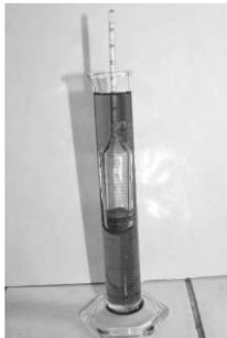
Fig. 1. Determination of oil density
