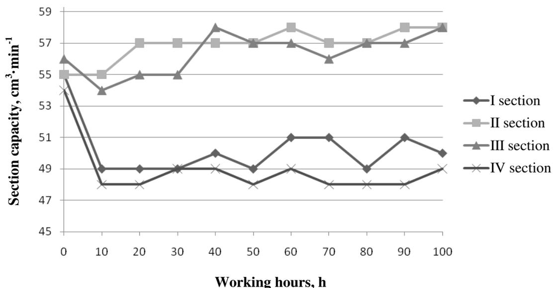
Fig. 3. Section capacity of injection pump depending on test time
