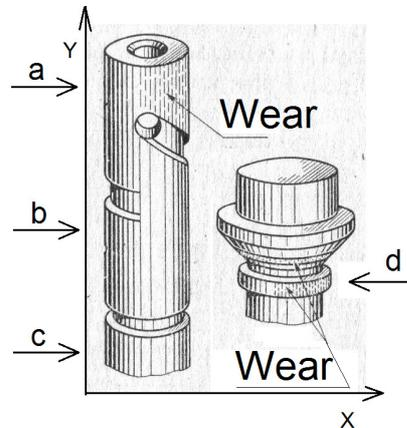
Fig. 1. Measurement methods for fuel injection pump parts [5]
