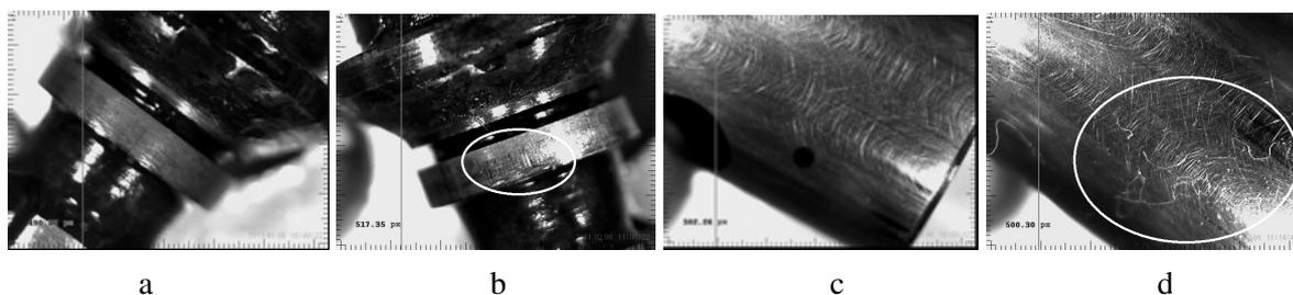
Fig. 5. Work surface of subsystem: a – unloading collar before testing; b – unloading collar after testing; c – pump plunger before testing; d – pump plunger after testing.
