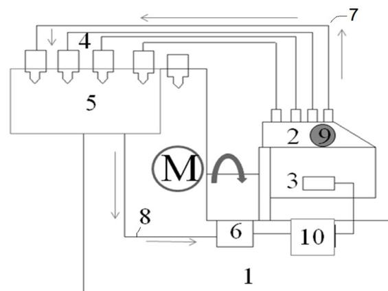
Fig. 2. Scheme of test principle: 1– stand; 2 – fuel injection pump; 3 – fuel pre-supply pump; 4 – injector; 5 – fuel container; 6 – cooling system; 7 – fuel injection pipes; 8 – fuel pre-supply pipes; 9 – thermometer; 10 – fine filter
