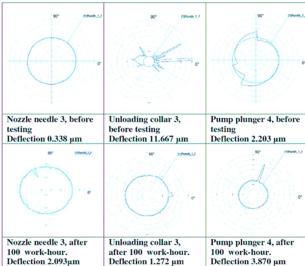
Fig. 4. Measurement results of geometric circularity of subsystem parts
