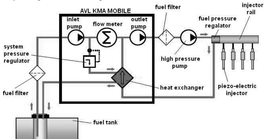
Fig. 2. AVL KMA Mobile fitting scheme [1]
