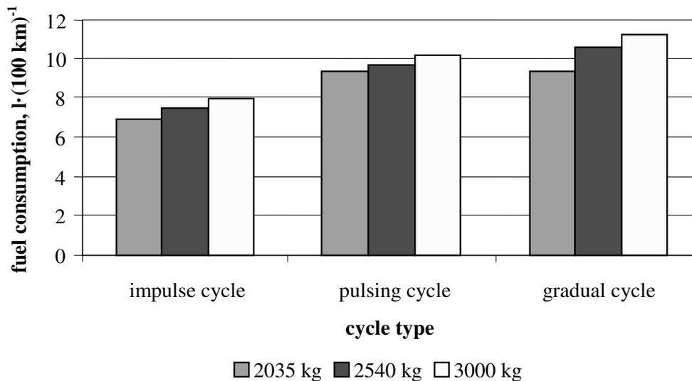
Fig. 6. Chassis dynamometer experiment results
