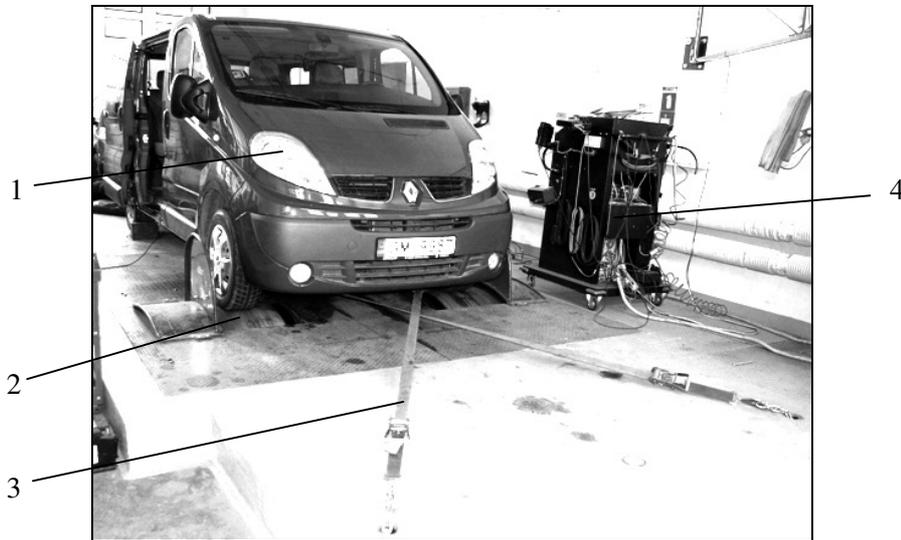
Fig. 3. Renault Traffic on chassis dynamometer: 1 – automobile; 2 – roll; 3 – straps; 4 – control platform
