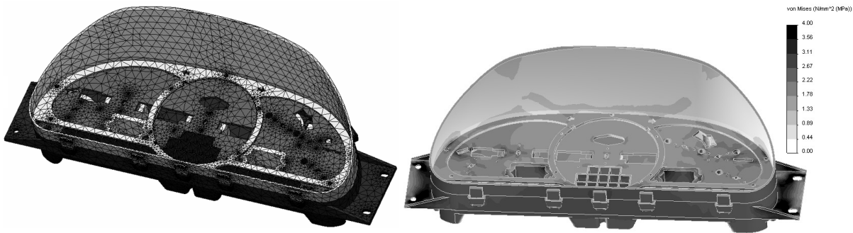
Fig. 2. Meshed 3D model and von Mises stresses distribution in initial design of GP
