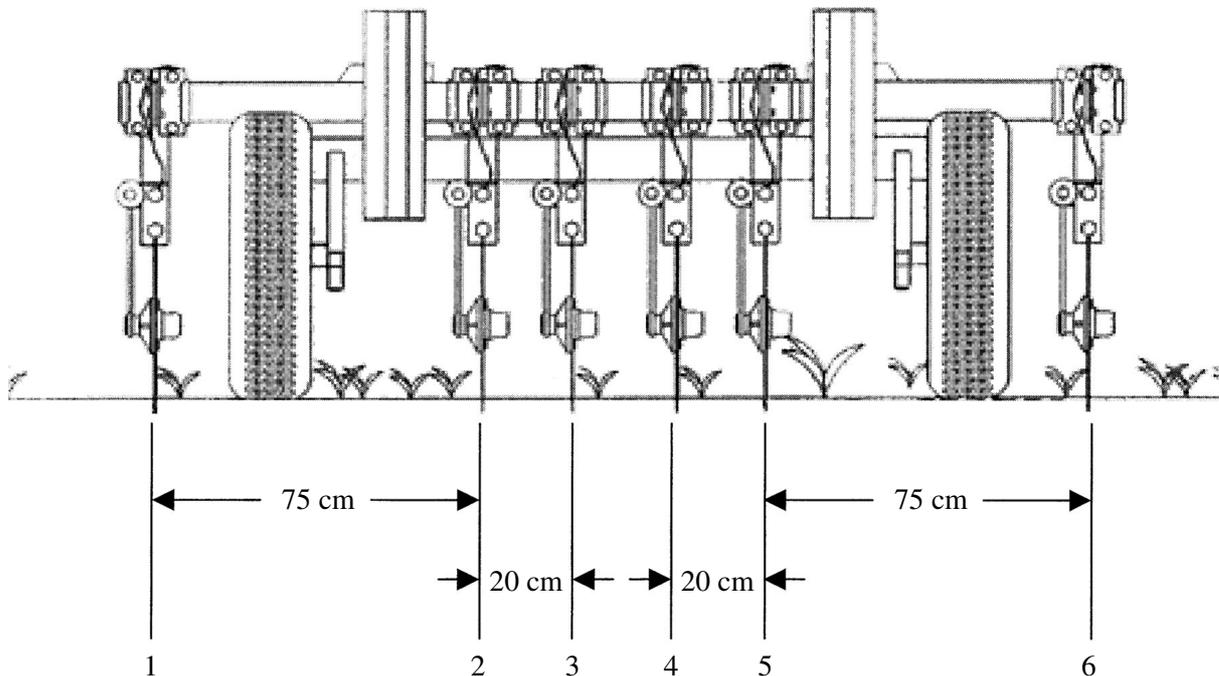
Fig. 1. Veris Technologies 3100 soil electrical conductivity (EC) mapping system: 2, 5 – voltage injector electrodes; 1,6; 3,4 – voltage drop measure electrodes; 1-2, 5-6 – deep soil profile; 2-3, 5-4, – shallow soil profile [3]
