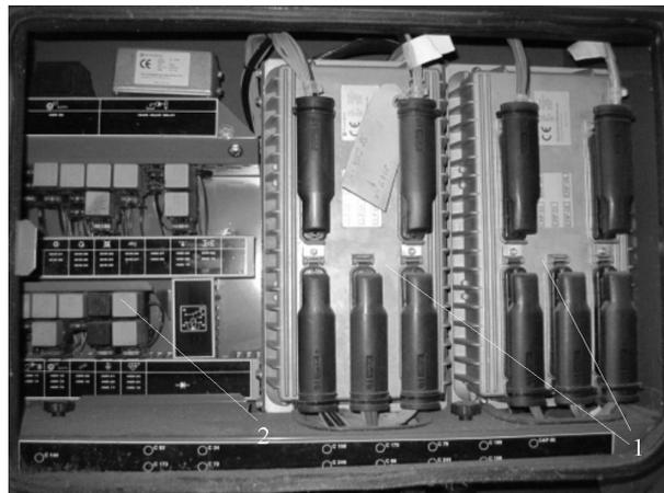
Fig. 3. **Control unit of harvesting thrasher:** 1 – control unit; 2 – relay block
