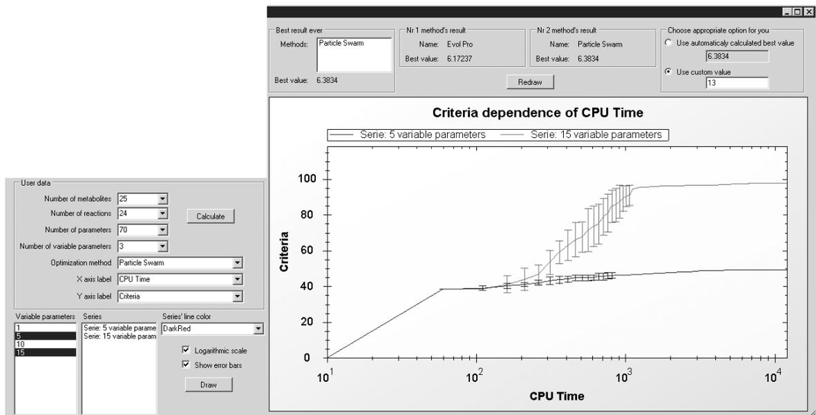
**Fig. 5. Comparison of variable parameter curves based on chosen input parameters and manually specified global optimum value**
